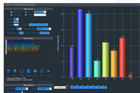
Surface fraction of material orientation in the vicinity of stable orientations of rolled IF steel
