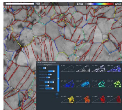
Grain boundaries disorientation and projection of the disorientation axis in titanium
