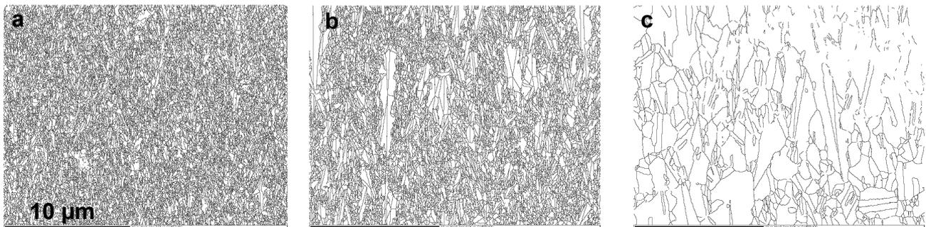
Fig. 1: EBSD grain boundary maps of PED nickel parallel to GD (vertical): (a) as-prepared state; (b) after annealing for 20 min at 350°C; (c) after annealing for 20 min at 600°C.
